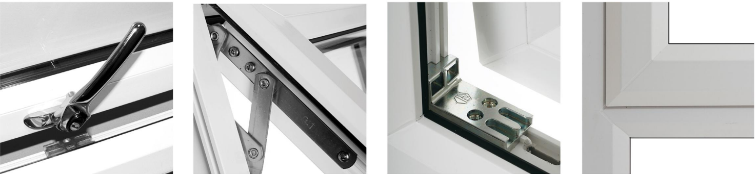
A range of key-lockable handles in offset, monkey tail and teardrop designs. Friction stays for smooth and reliable operation all year round. Window keeps with dual slots enabling a lockable 'slightly-ajar' ventilation position. Close-up of fusion-welded sash corner and mid-rail overlap.
